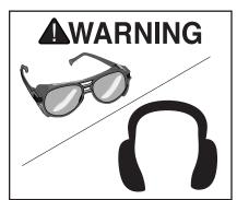
Operating this nailer can propel objects into the air, causing immediate eye damage. To protect yourself, always wear American National Standards Institute (ANSI) approved safety glasses or goggles when operating this equipment. In addition, this nailer discharges at up to 85-90 decibels. To protect your hearing, always wear ANSI approved ear protection when operating this nailer.
